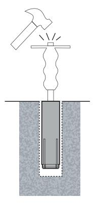
Use a manual expansion tool for drop in anchors.
